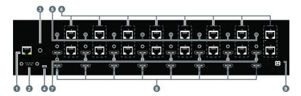
**1CONTROL**: This port is the link for Telnet control, connect to an active Ethernet link with an RJ45 terminated cable (for further details, please refer to sections 6.8 and 6.9).
